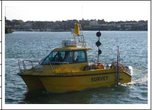
During the survey, the vessel will display the prescribed lights and day shape signals for the operations being completed and will be monitoring VHF Channel 16.
